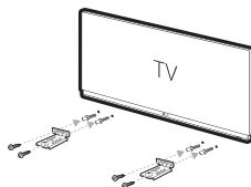
5. Put the unit on the brackets to match screw holes on the bottom of the unit.
