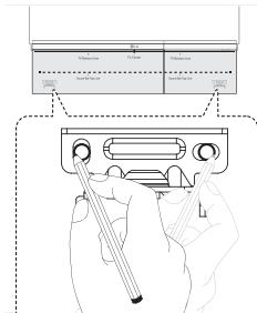
3. Remove the Wall bracket install guide.
