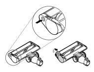
3 Pull the brush cover forward and pull the main brush out.
