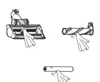
7 Slide the brushes back into the nozzle and rotate the cover back into place. Turn the cover lock clockwise to lock the cover.
