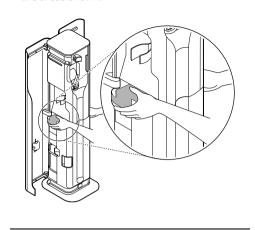
2 Open the right door and insert the combination tool 2 and the crevice tool 3 for storage.
