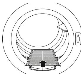
**3** Insert the front of the dryer rack into the hole next to the lint filter and press it to complete assembly.
