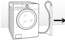
Connecting the drain line
