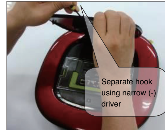
3. Separate center hook (Be careful not to break)
