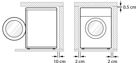
**Level floor** : Allowable slope under the entire appliance is 1°.
