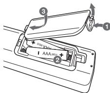
Remove the battery cover on the rear of the Remote Control, and insert two (size AAA) batteries with **+** and **–** matched correctly.
