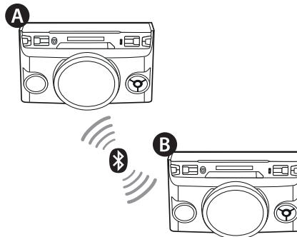
1. Press and hold **F / WIRELESS LINK** on the unit for 3 seconds. PARTY LINK MODE SELECT appears in the display window.
