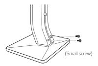
2. Secure the connection with a supplied screw, then insert a speaker wire from the bottom of the base.
