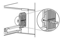
Press on the hooks on the deodorizer and remove it.
