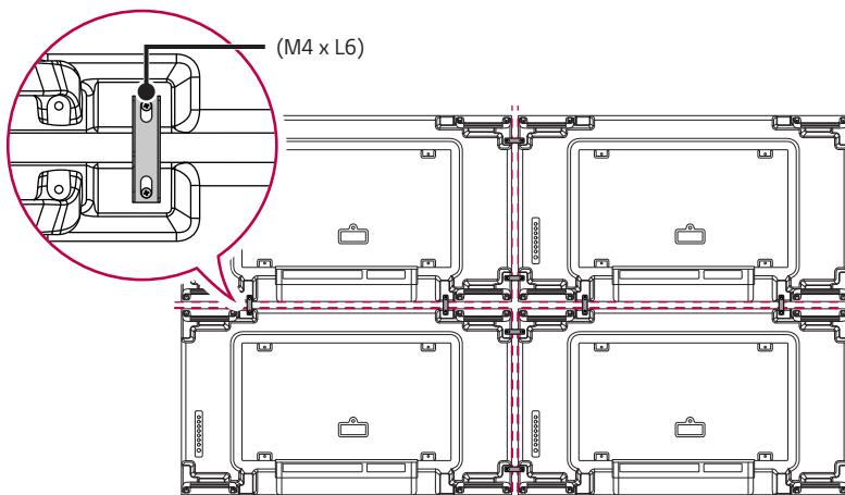
2 Adjust the spacing between the sets using the tiling guide, and remove the protective sheet.
