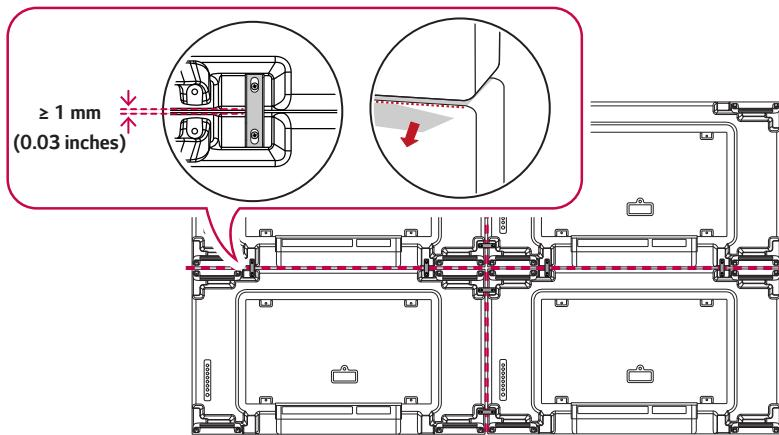
3 Complete the  $2 \times 2$  tiling. You can use various options of tiling including  $3 \times 3$  by using the same method.
