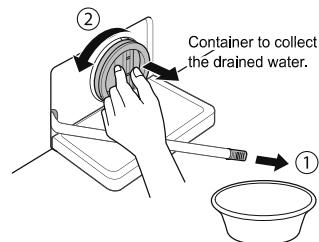
3 Remove any extraneous matter from the pump filter.
