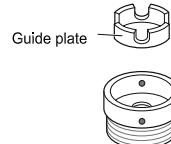
**3** Push the adapter onto the end of the tap so that the rubber seal forms a watertight connection. Tighten the four fixing screws and the adapter ring plate.
