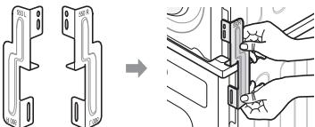
**4** Fasten the 2 screws that were removed earlier from the appliance to the stacking kit.
