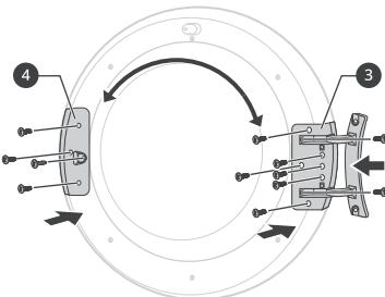
**5** Remove the door catch ❸ from the appliance frame by removing 2 screws and then assemble them on the opposite side.
