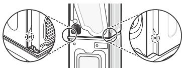
**3** Align the LG stacking kit holes and the rear cover holes in a line.
