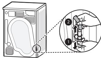
**2** Attach the anti-backflow lid **1** to the head of the connecting elbow or T piece and then connect the optional drain hose **3** to the opposite side of the connecting elbow or T piece.
