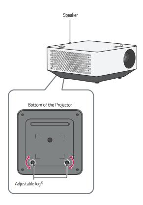
1) Turn the adjustable leg left or right to adjust the angle.
