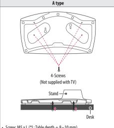
• Screw: M5 x L (\*L: Table depth + 8~10 mm) ex) Table depth: 15 mm, Screw: M5 x L25
