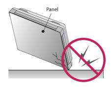
If the product is tilted onto the edge of the panel, the panel may be damaged.
