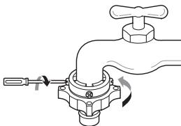
4 Pull the connector latch plate down, push the supply hose onto the adapter, and release the connector latch plate. Make sure the adapter locks into place.
