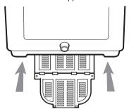
Insert the 2 screws into the holes to assemble the anti-rat cover to the appliance.
