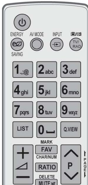
**POWER** Switches the TV on from standby or off to standby.
