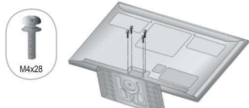
When assembling the stand, make sure to distinguish and assemble the front and rear side of the stand correctly.
