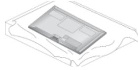
2 Set the **Stand Base** on even floor. Assemble the parts of the **Stand Body** with the **Stand Base** of the TV.
