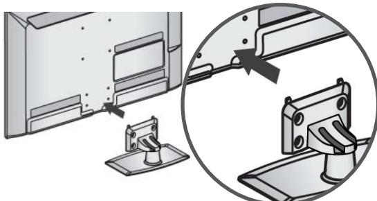
4 Assemble the parts of the **Stand Rear Cover** with the TV.
