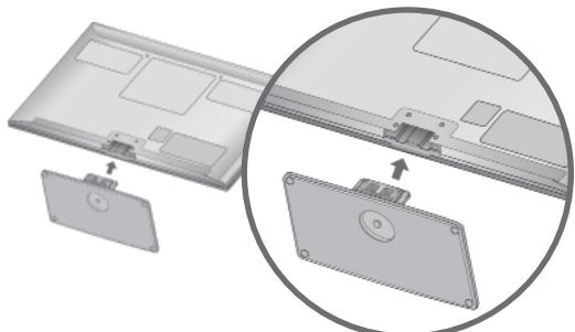
5 Fix the 4 bolts securely using the holes in the back of the TV.
