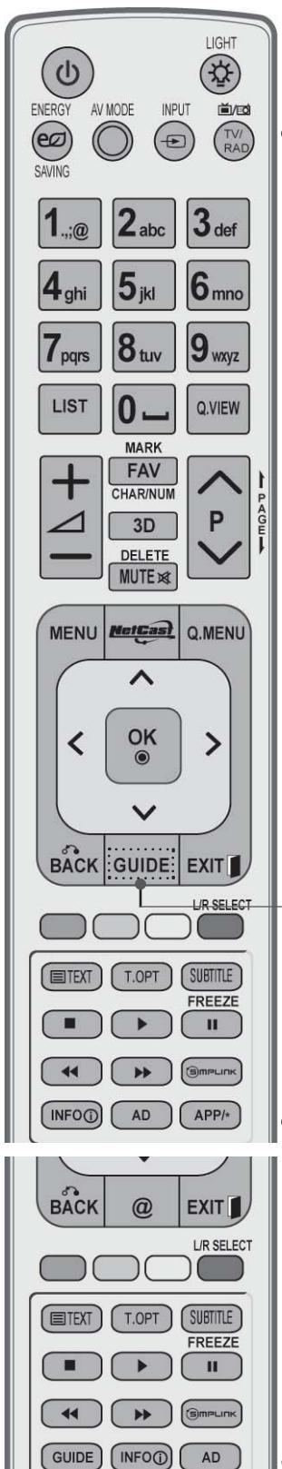
POWER (POWER) Switches the TV on from standby or off to standby.
