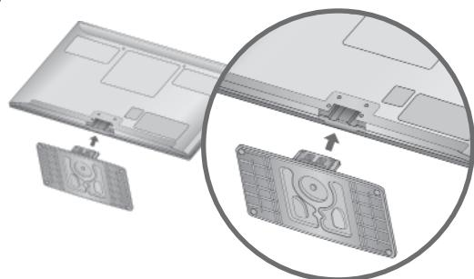
4 Fix the 4 bolts securely using the holes in the back of the TV.
