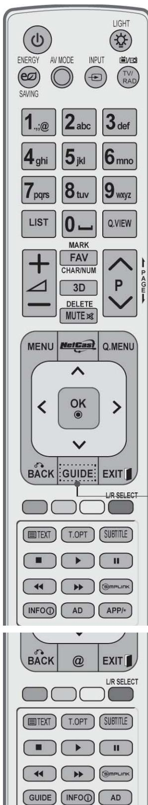
**POWER** Switches the TV on from standby or off to standby.
