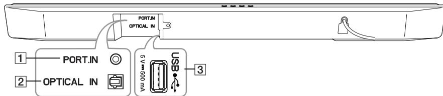
**[1] PORT.IN** : Connect to a Portable device.
