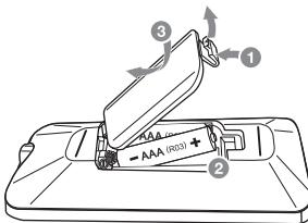
Remove the battery cover on the rear of the remote control, and insert battery with  $\oplus$  and  $\ominus$  matched correctly.
