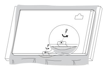
2 After removing the screw, remove the LG Logo Bracket. Attach the LG Logo Bracket with a screw, aligning it with the hole on the right side.
