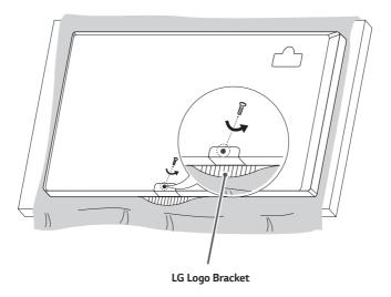
2 After removing the screw, remove the LG Logo Bracket. When re-attaching the LG Logo Bracket, repeat the process in reverse order.
