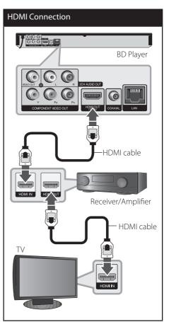
Connect the amplifier's HDMI output jack to HDMI input jack on your TV using a HDMI cable if your amplifier has HDMI output jack.
