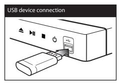
When you connect the USB device on the HOME menu, the player plays a music file contained in the USB storage device automatically. If the USB storage device is containing various types of files, a menu for the file type selection will appear.
