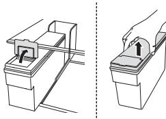
3 Fill with bottle filtered or clean filtered water up to the reference line indicated inside the water dispenser tank. (Total capacity: 4 l)
