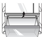
2 Insert the bottom of the vegetable drawer into its original position and gently push it back in while lowering it.
