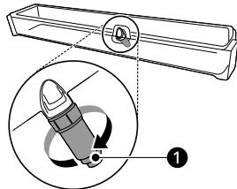
4 Hold the lever of the ice tray and turn it clockwise to release the ice cubes.
