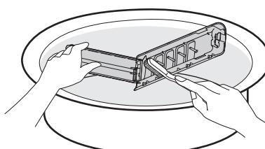
**4** Close the lid and then insert the lower part of the filter into the wash drum. Press the top of the filter until you hear a **click sound**.
