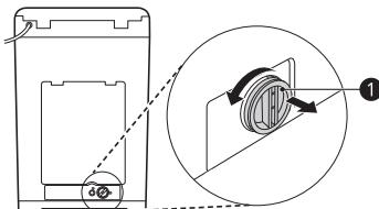
6 Remove any foreign objects and fluff inside pump casing and from the filter.
