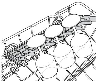
The left side row of tines can be folded down or the cup racks can be folded up out of the way for tall crockery items.
