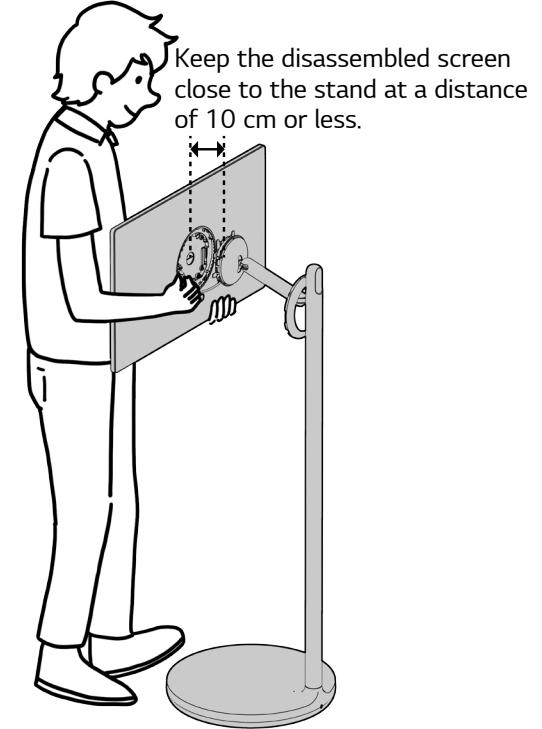
7 Press the plug lock, push it in the direction of the arrow, and then disassemble the screen completely.
