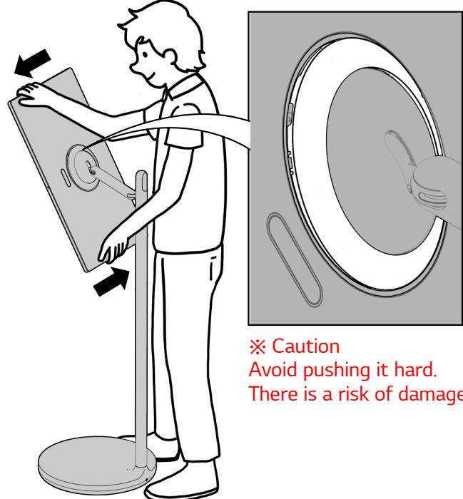
3 Use a wedge or pull it with your hand to completely disassemble the cover.
