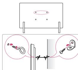
1 Insert and tighten the eye-bolts, or TV brackets and bolts on the back of the TV.
