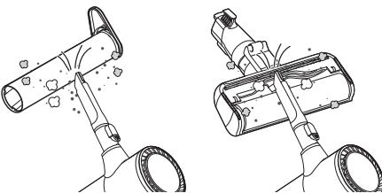
4 Use a damp towel or cloth to remove any remaining foreign objects and dust from the brush and the bottom of the nozzle. Remove foreign objects, debris and hair from all Rollers of the nozzles using tweezers.
