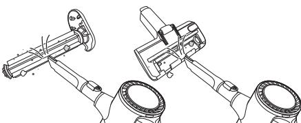
4 Use a damp towel or cloth to remove any remaining foreign objects and dust from the brush and the bottom of the nozzle. Remove foreign objects, debris and hair from all Rollers of the nozzles using tweezers.
