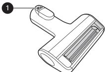
2 Remove the rotating brush while holding down the **PUSH** button on the nozzle.
