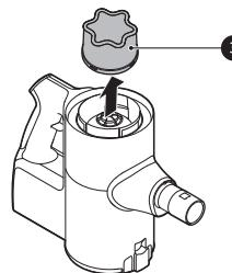
**4** Use the combination tool **4** to clean any dust off the motor.
