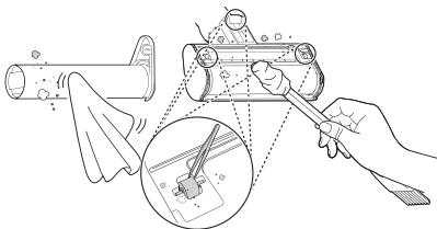
6 Slide the brush back into the nozzle and rotate the cover back into place. Turn the cover lock clockwise to lock the cover.
