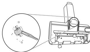
5 Insert the left side of the brush ② into the groove ③ inside the nozzle.
