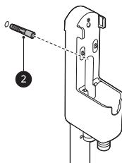
**7** Align the wall anchoring block **③** of the charging station, and fix the charging station
