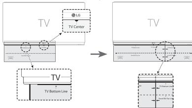
2. When you mount it on a wall (concrete), use the wall plugs. You should drill some holes. A guide sheet (Wall bracket install guide) is supplied to drill. Use the sheet to check the point to drill.
