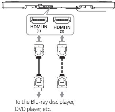
1. Connect HDMI IN (1) or HDMI IN (2) jack on the back of the unit to HDMI OUT jack on the audio device such as Blu-ray disc player, DVD player, etc.
