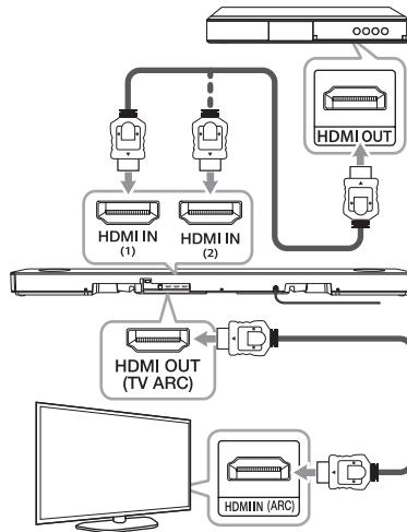
1. Connect HDMI IN (1) or HDMI IN (2) jack on the back of the unit to HDMI OUT jack on the external device such as Blu-ray disc player, DVD player, etc.
