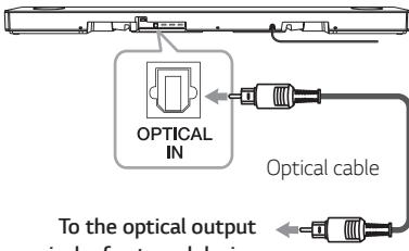
1. Connect the OPTICAL IN jack on the back of the unit to optical out jack of your external device.
