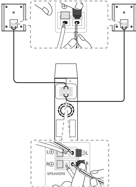
2. Connect the wireless receiver and the rear speakers (right, left) with the speaker cables.
