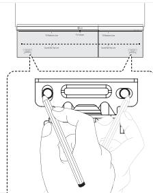
3. Remove the Wall bracket install guide.
