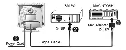
NOTE: For Apple Macintosh use, a separate plug adapter is needed to change the 15 pin high density (3 row) D-sub VGA connector on the supplied cable to a 15 pin 2 row connector.
