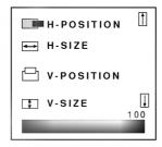
The bar graph shows you the current level of the selected "H-Position" control. Use the Adjustment control knob to increase or decrease the level to fit the screen or your desired size. When you have finished, press the Enter (→) button once to return to Main Menu1 to make another selection. If you have completely finished using the OSD after you have returned to Main Menu1, you can double Click the Enter button to exit the OSD.
