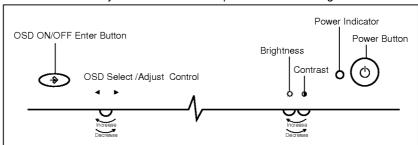
Buttons on the front of the monitor allow you to adjust image easily through an OSD menu. As you choose controls, the selected icon shows you what the chosen control will do. These pictures give you immediate understanding of the controls. The following is a description of use for each button.
