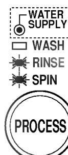
Process indicator lamp flickers (Rinse, Spin) when draining does not take place.
