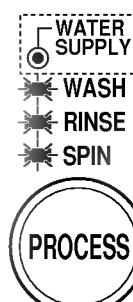
Process indicator lamp flickers (Wash, Rinse, Spin) when tub does not spin.
