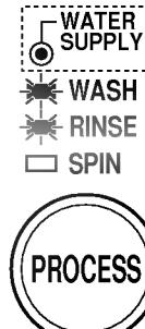
Process indicator lamp flickers (Wash, Rinse) when water does not flow into the tub.
