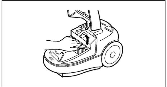
2. Brush up dust and wash filter in a warm soapy water. Do not clean in a dish washer or in a washing machine.
