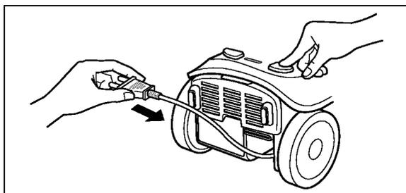
5. Always pull out the power cord by holding the plug, not the cord.
