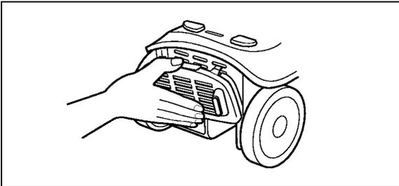
2. Replace the old micro filter with the new micro filter. Be sure to fit the guide rib of the rear cover and the holes of micro filter.
