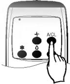
(Operation will start when the Button is pressed, and stop when the button is pressed again.)
