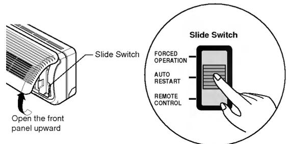
*When you are out for a while, move the Slide Switch to the REMOTE CONTROL.*
