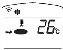
For more fresh feeling than other fan speed, press the Indoor Fan Speed Selector and set to CHAOS mode. In this mode, the wind blows like natural breeze by automatically changing fan speed according to the CHAOS logic.
