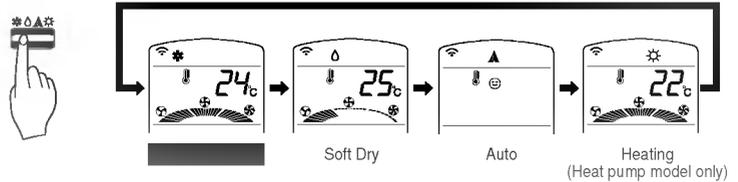
3 Close the door on the remote control. Set the temperature lower than the room temperature. The temperature can be set within a range of 18°C~30°C in 1°C increments.
