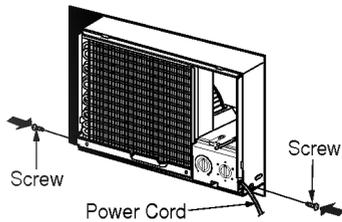
**CAUTION:** The power cord must be connected to an independent circuit. The green wire must be grounded.
