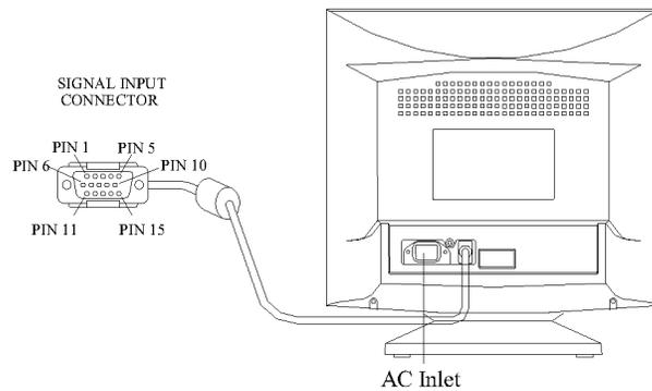
Figure 2 Connecting Cables
