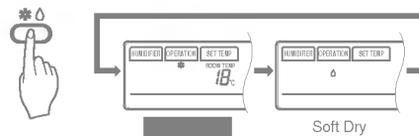
3 Set the temperature lower than the room temperature. The temperature can be set within a range of 18°C~30°C in 1°C increment.
