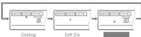
3 Set the temperature higher than the room temperature. The temperature can be set within a range of 16°C~30°C in 1°C increments.
