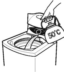
**3** Submerge the separated hose in 50°C of hot water
