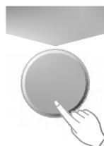
**3** Press both the **WATER TEMP.** key and the **WATER LEVEL** key simultaneously while wash is proceeding, then all the keys are locked until completing the wash program or unlocking them.
