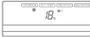
• The temperature can be set within a range of 18°C ~ 30°C by 1°C.
