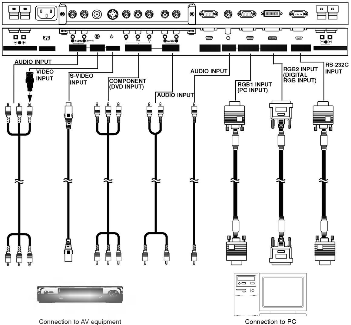
**Note :** All cables shown are not provided with the Monitor, except : A D-sub 15 pin cable and DVI cable is supplied to connect the Monitor to a PC.
