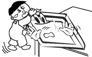
**There should be enough distance between an outside antenna and power lines to keep the former from touching the latter even when the antenna falls.**
