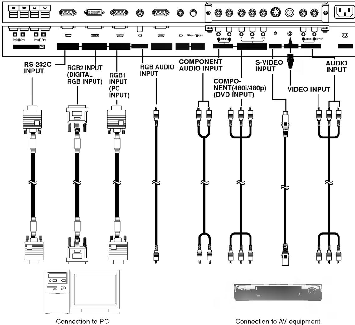
**Note:** The connection cables shown above to the right are not included with the Monitor.
