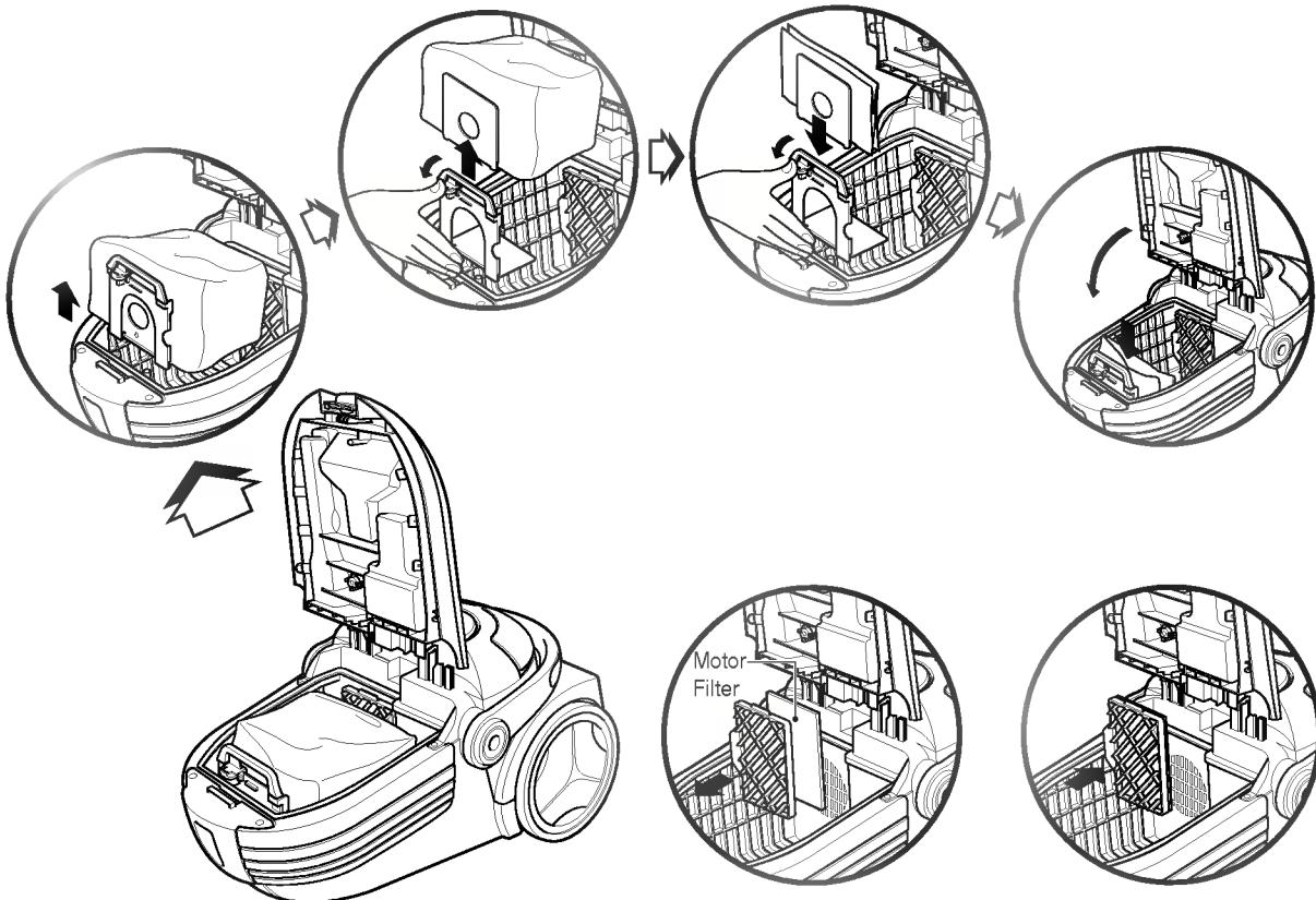
The dust bag needs changing when the cleaner is set to maximum power and the cleaner head is off the floor but the "bag full" indicator window is completely coloured red.
