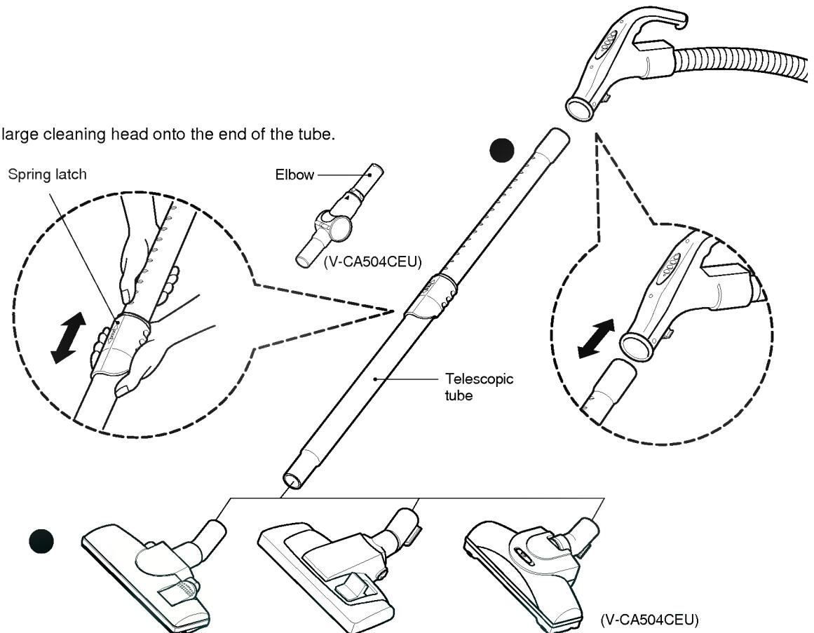
Push telescopic tube into nozzle outlet.
