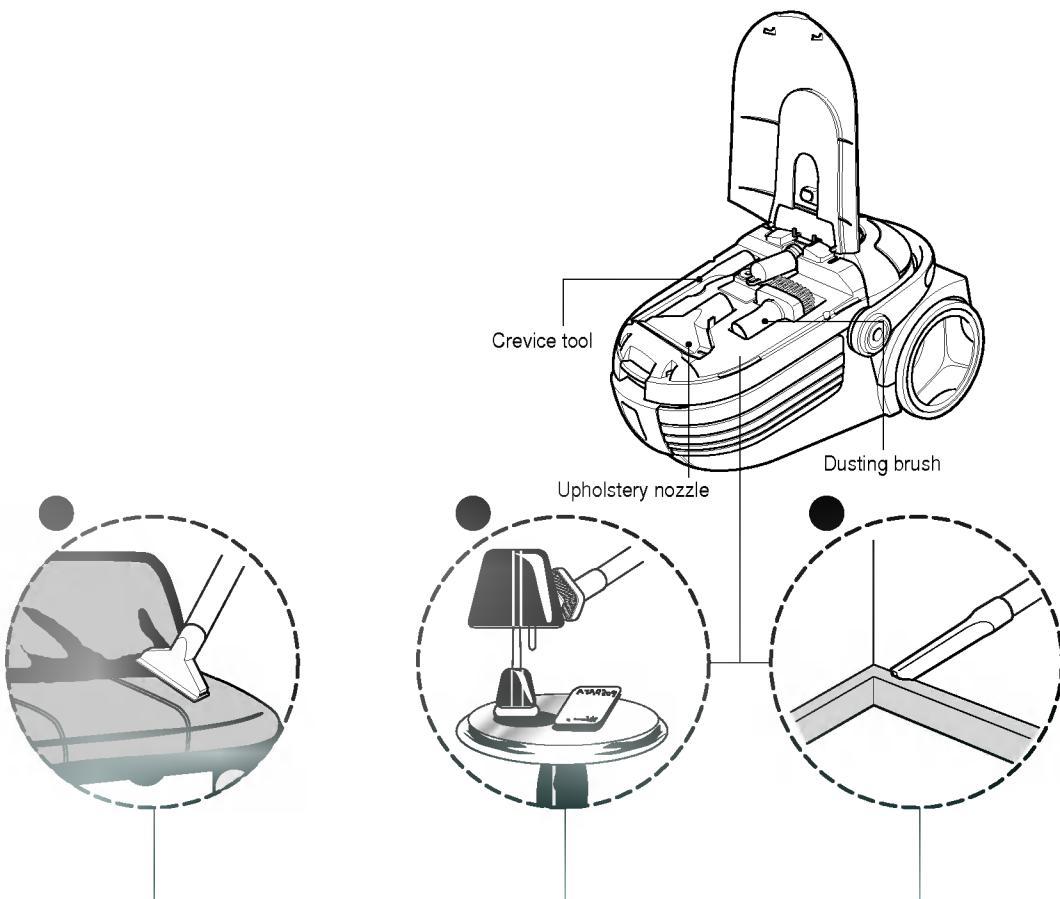
Upholstery Nozzle is for vacuuming upholstery, mattresses, etc. The thread collectors help to pick up the threads and fluff.
