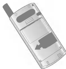
To remove the SIM card
