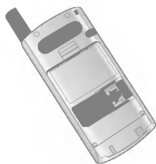
To insert the SIM card
