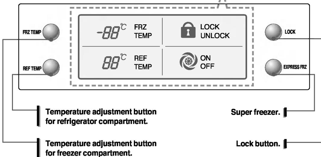
You can adjust temperature of and freezer room and refrigerator room.
