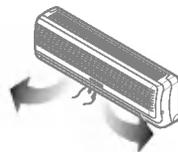
Adjust the left/right airflow direction by hand.
