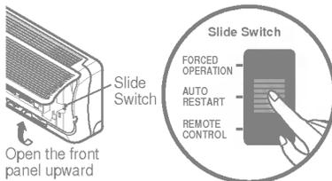
When you are out for a while, put the Slide Switch on the Remote Control.
