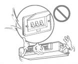
Install the panel and the cover of control box securely.
