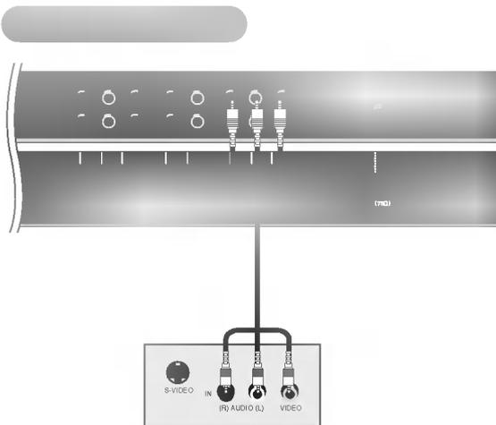
The TV has a special signal output capability which allows you to hook up a second TV or monitor.
