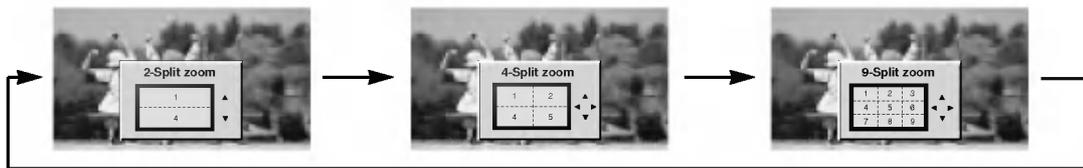
2. Press the number button corresponding to the section you wish to enlarge. You can move within the enlarged picture using the **▲ / ▼ / ◀ / ▶** button. To return to normal viewing, press the **SPLIT ZOOM** button again.
