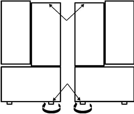
3. Open both doors again and check to make sure that they close easily. If not, tilt the refrigerator slightly more to the rear by turning both leveling screws clockwise. It may take several more turns, and you should turn both leveling screws the same amount.
