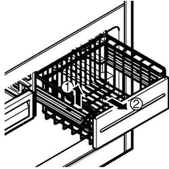
2. To Install, pull both rails out to full extension. Hook the basket supports into the rail tabs and push to the back of compartment.
