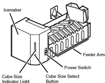
The icemaker will produce eight cubes per cycle—approximately 100–130 cubes in a 24-hour period, depending on freezer compartment temperature, room temperature, number of door openings and other operating conditions.
