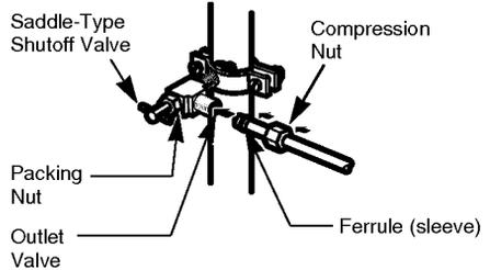
**NOTE:** Commonwealth of Massachusetts Plumbing Codes 248CMR shall be adhered to. Saddle valves are illegal and use is not permitted in Massachusetts. Consult with your licensed plumber.
