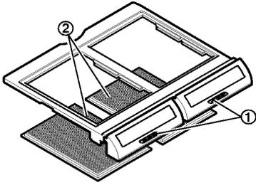
The Optibin Crispers provide fresher-tasting fruit and vegetables by letting you easily control humidity inside the crisper. The Optibin Crispers include: 1) a humidity control knob at the front of the crisper cover and 2) a large lattice on the inner surface of the cover to hold or release moisture.
