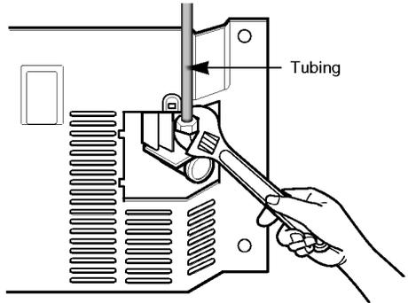
**▲ CAUTION:** Check to see if water dripping occurs at water line connections.
