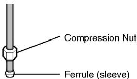
4. Insert the tube into the valve and fasten with wrench as shown in the figure below.
