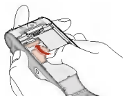
To insert the SIM card
